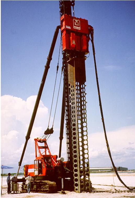
**Figure 8.** Resonance compaction machine with flexible, double-Y compaction probe at Map Ta Phut, Thailand (source: Massarsch and Westerberg, 1995a)
